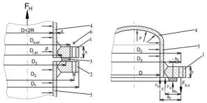
Fig. 1. Flat flange joints of the integral type 1, 2 – flanges; 3 – sealing gasket; 4, 5 – shells; 6 - bolts.
